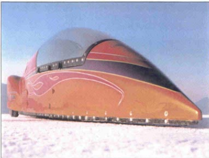
This nose shot shows how close the Flatfire is to the ground in an effort to maximize its aerodynamics.
