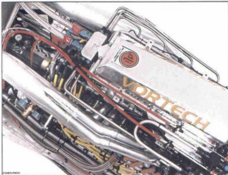
Beneath all of this high-tech equipment rests a 1946 Ford flathead engine that originally cranked out only 100 hp; it now produces over 700 hp.
